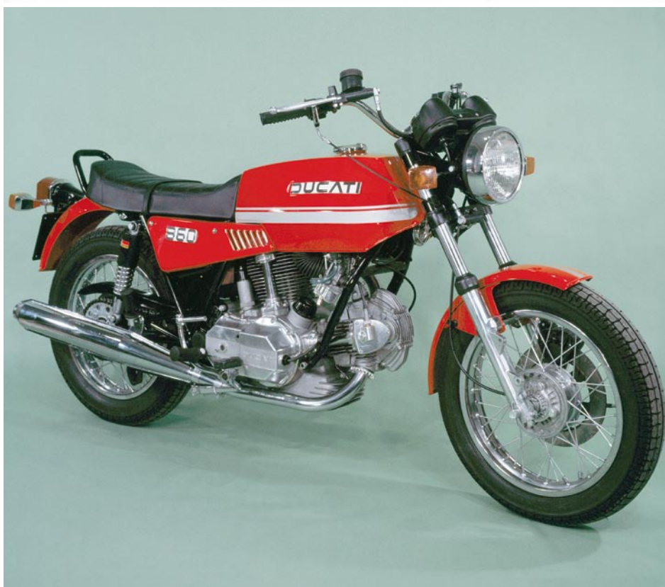
Another publicity picture of the 860 GT with the lower seat, this time with a single front disc brake. (Courtesy Ducati Motor)
