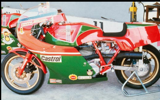
The 1979 factory F1 bike featured a box-section swingarm and special exhaust. This was the first form, as it appeared at the test at Misano. (Courtesy Ducati Motor)
